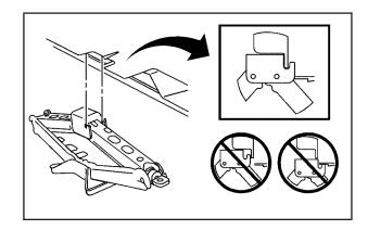
Raise the jack by turning the wheel wrench clockwise until the slots in the jack head fit into the metal flange located behind the triangle on the plastic molding as shown.
